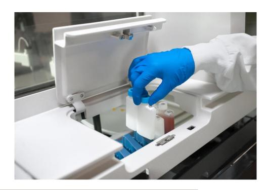
**NOTE:** Opening the reagent tray drawer during the loading process halts the loader and moves the reagent tray back to the loading area.
