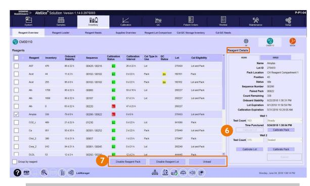
**NOTE:** Disabling a reagent pack with a paired reagent pack on another CH analyzer server disables both reagent packs.
